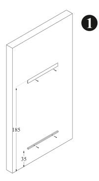
Carier is mounted on the wall with specified dimension
