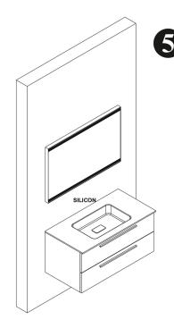
Fill up silicon between the bench and well.
